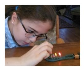
Play Doh circuits. Commercial Play Doh conducts electricity. You will need play doh, small LEDs, and a 9-volt battery (also experiment with other batteries). Make "wires" out of rolled-out play doh and also incorporate lights in creative sculptures. What affects the brightness of the LEDs? These photos show the creation of both a parallel and a series circuit. For ideas, see
