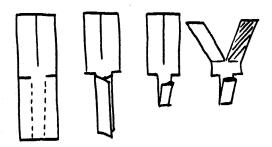
Paper Helicopters. Make paper helicopters and drop them from as high as you can reach; e.g., off a step stool or perhaps playground equipment. A good design is made from a fourth of a sheet of paper (cut the paper in four strips across the sheet). Fold the helicopter as shown on the drawing. Paper clips can be added to experiment with how they affect the helicopter's flight.
